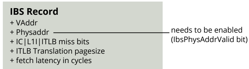
Figure 3.2: Fetch record. When a certain amount of events has passed, one instruction is sampled in detail. The IBS record contains all information valuable to the programmer, such as miss addresses, miss information bits, and fetch latencies [1].
