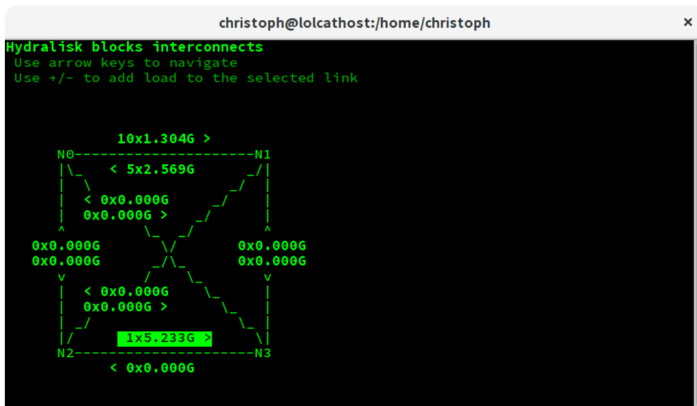
Figure 4.11: Hydralisk. The command-line interface presents the topology of the test platform (limited to four-node configurations currently) to the user. Engineers are able to select each unidirectional QPI channel and add bandwidth load. In this case, the QPI link between node 0 and node 1 is loaded in a bidirectional fashion. The channel from node 2 to 3 is loaded with one instance of stream triad only, which does not suffice to reach the channel's capacity.
